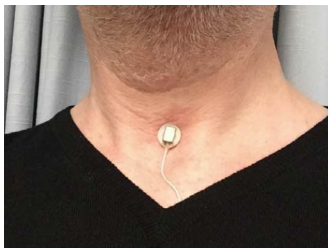
Figure 1. Accelerometer attached to the skin on the tracheal wall.
